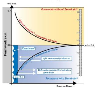
With Conventional formwork, air and excess water in the concrete are expelled to the formwork surface by vibration energy. The result is blowholes, other surface blemishes, an increased w/c ratio and decreased cement content in the concrete cover zone. It is easier and quicker for harmful substances to penetrate this more porous concrete. Aggressive agents can begin their destructive work earlier and more intensively.
