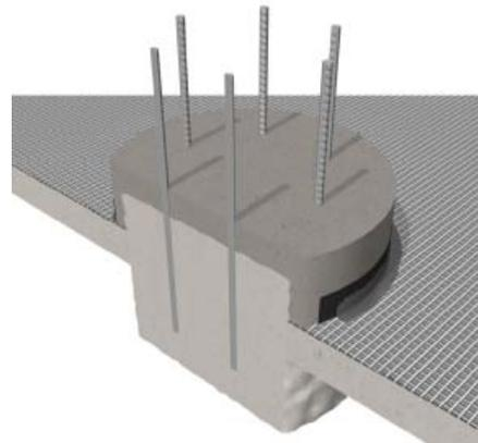
**Epoxy grout encapsulating the pile top and flowing into the Proofex Engage mesh to give assured watertight integrity in deep basements. Finished off with a seam of Polyurea WCS.**
