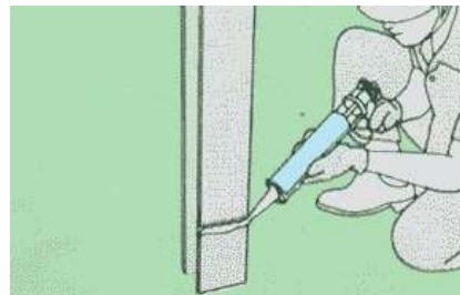
5. Apply Leakmaster continuously without a break to the place to be sealed.
