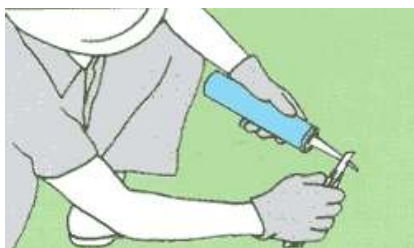
2. Cut the nozzle at the appropriate position diagonally.
