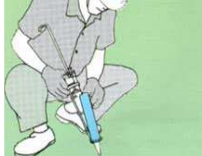
4. Set the cartridge to the caulking gun.
