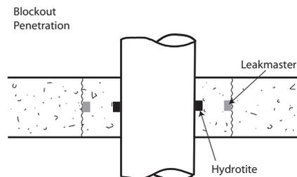
When thin walled PVC pipes are used there is a possibility the PVC pipe may bend inward due to the expansion pressure of Hydrotite. It is not recommended using less than 5 mm wall thickness PVC pipes.
