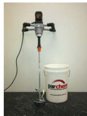
Typical grout mixing equipment
